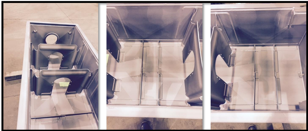
Figure 29: Final Oil Pan with Additional Stiffness and Support in Key Areas
