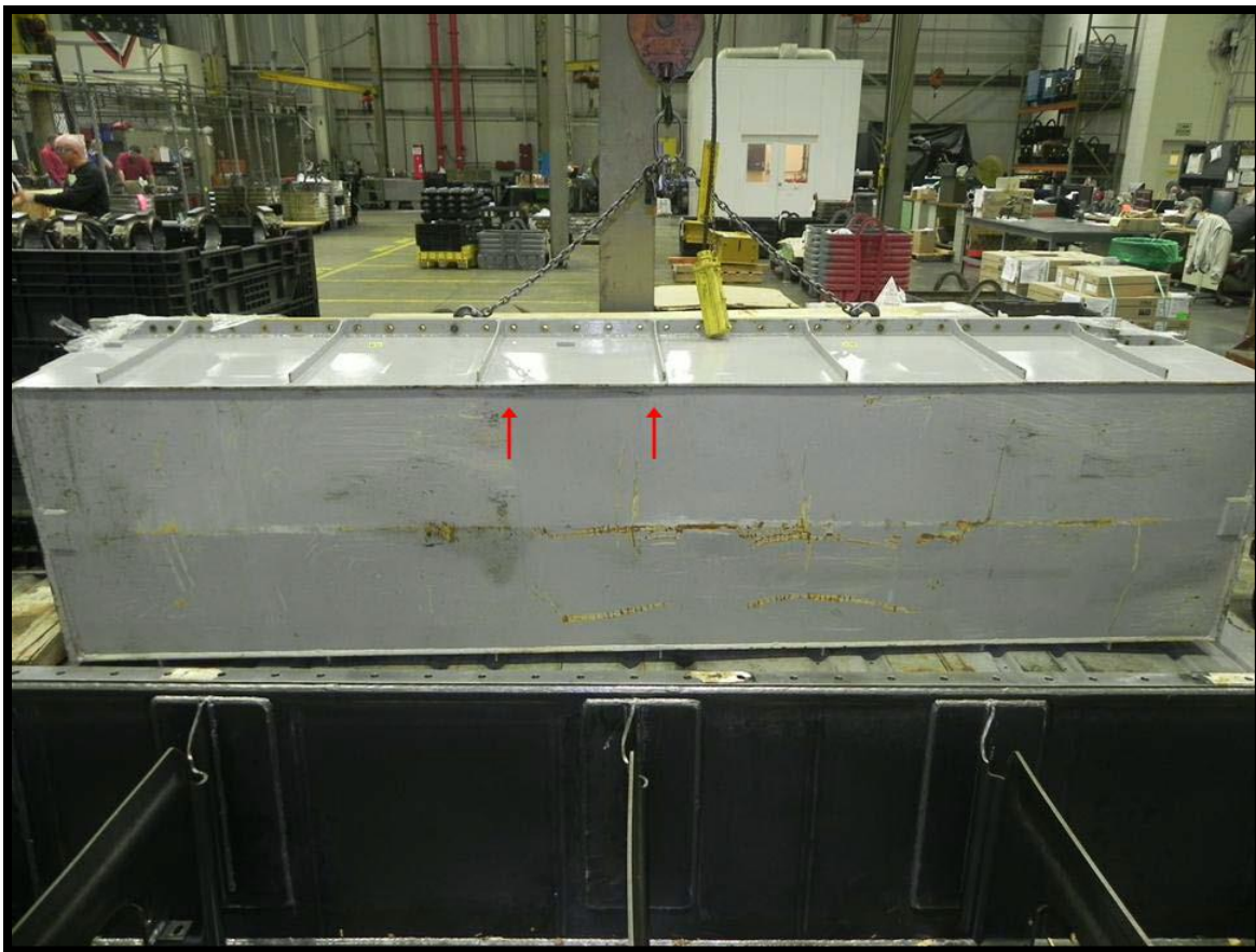
Figure 2: Crack on the Bottom of the Oil Pan
